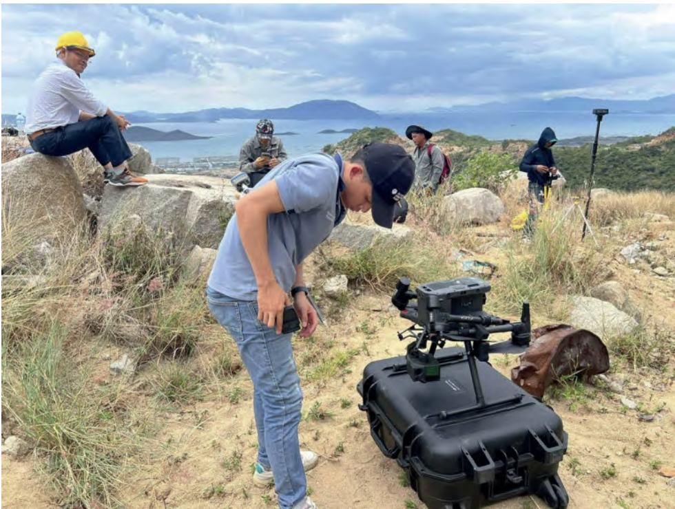
Site survey using LiDAR aerial imaging technology, 500kV transmission line Van Phong - Binh Dinh project
